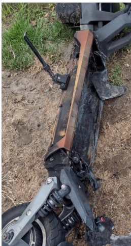
A tenants E-scooter after a battery explosion
