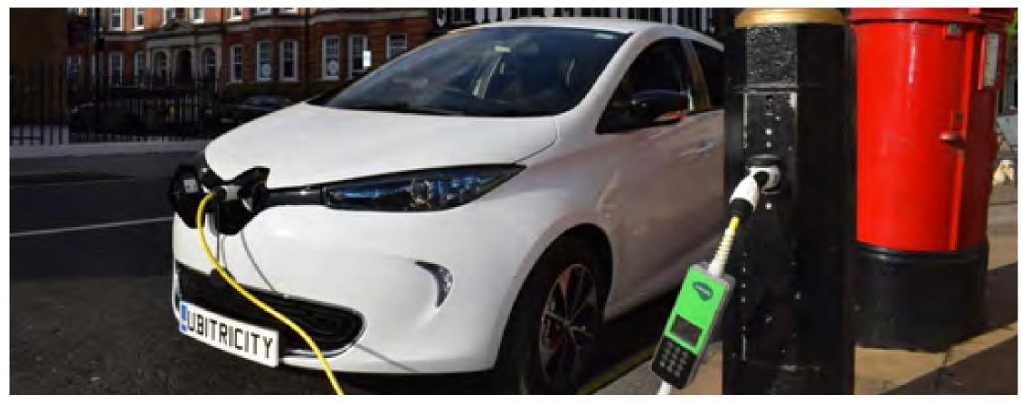
Figure 60. Electric charging point integrated with street furniture.
