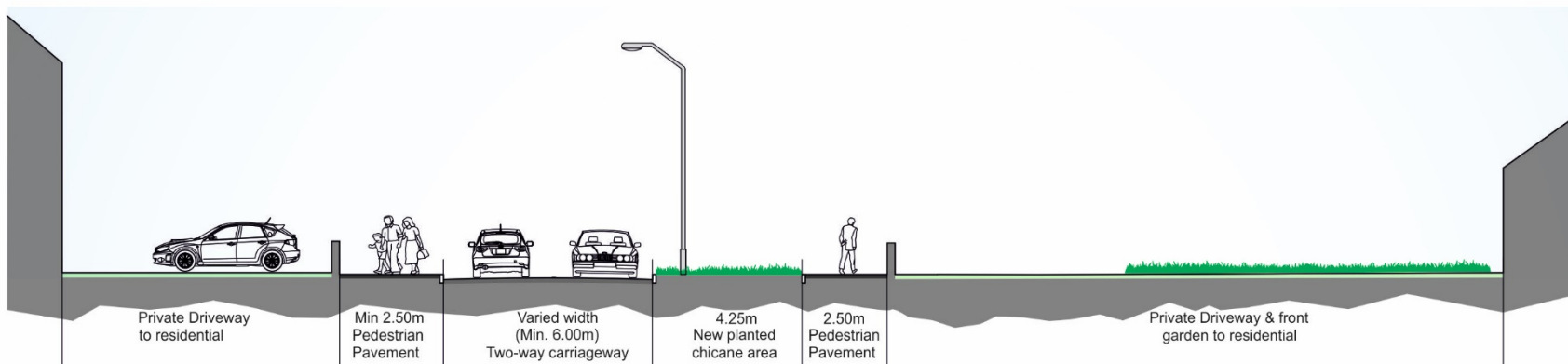
AREAS B - PROPOSED TYPICAL NEW CHICANE SECTION - VILLAGE ENTRANCE - 20MPH
